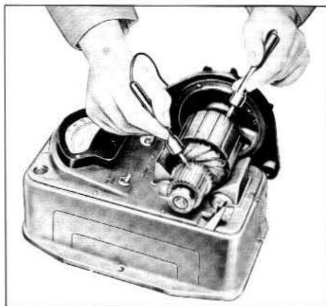
Fig. 10A-9—Testing Armature for Short Circuit to Shaft (60C-7668)
