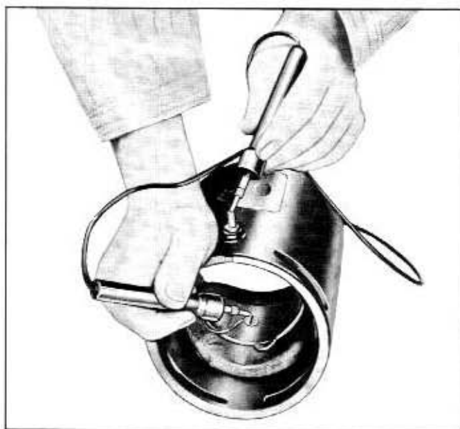
Fig. 10A-10—Testing Field Coils for Open Circuit—(60C-7669)
