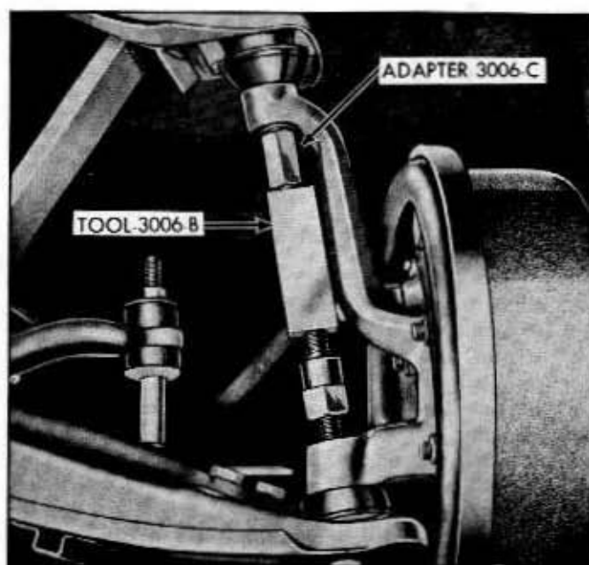
Fig. 3A-13—Ball Joint Expanding Tool—Installed—(60C-413)
