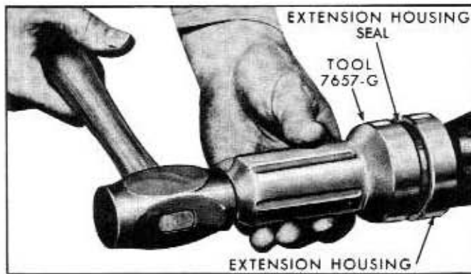
Fig. 7B-12—Installing Extension Housing Seal—(60C-4415)
