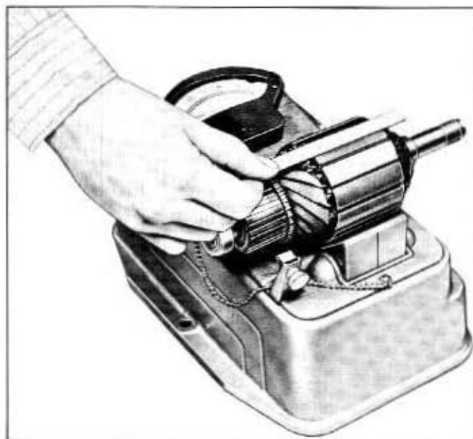
Fig. 10A-8—Testing Armature Windings for Short Circuits (60C-7667)
