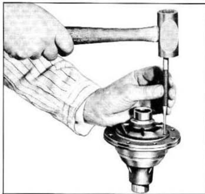
Fig. 4-21—Differential Pinion Shaft Retainer Removal—(60C-5212)
