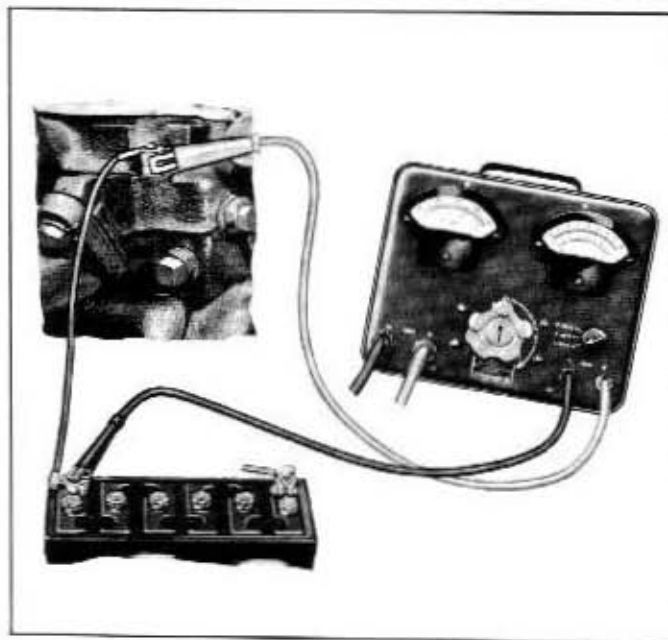
Fig. 10A-24—Connections for Negative Battery Cable Resistance Test—(60C-7682)
