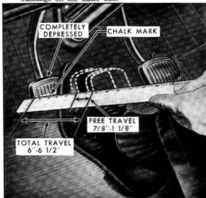
Fig. 7C-3—Checking Clutch Pedal Travel—Typical—(60C-3203)
