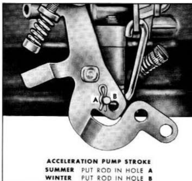
Fig. 9C-9—Accelerating Pump Stroke Adjustment—(60C-6822)
