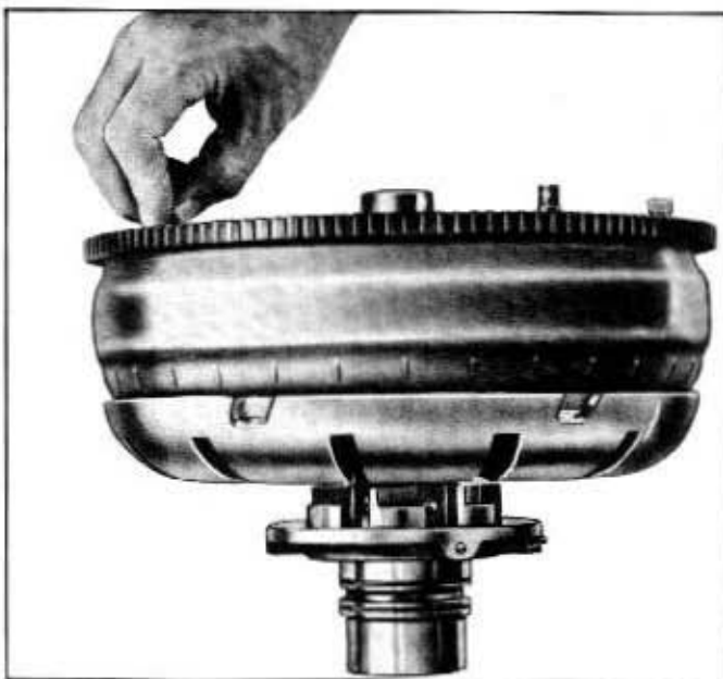
Fig. 7A-45—Stator to Impeller Interference Check—(60C-4445)
