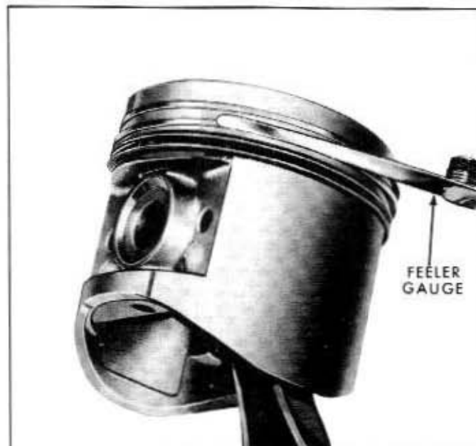
Fig. 6A-44—Checking Ring Side Clearance—Typical—(60C-5644)
