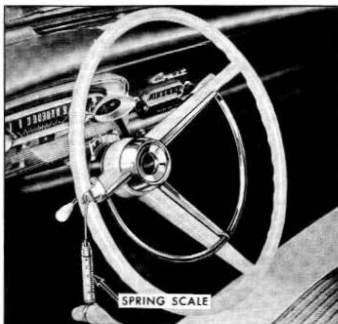
Fig. 3B-2—Steering Gear Load Check Using Pull Scale—Typical—(60C-1214)
