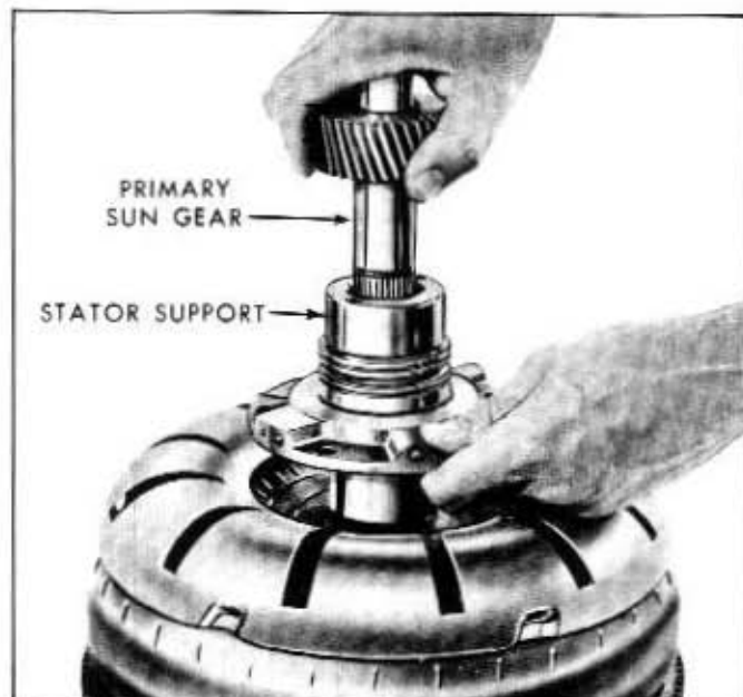
Fig. 7A-46—Stator to Turbine Interference Check—(60C-4446)
