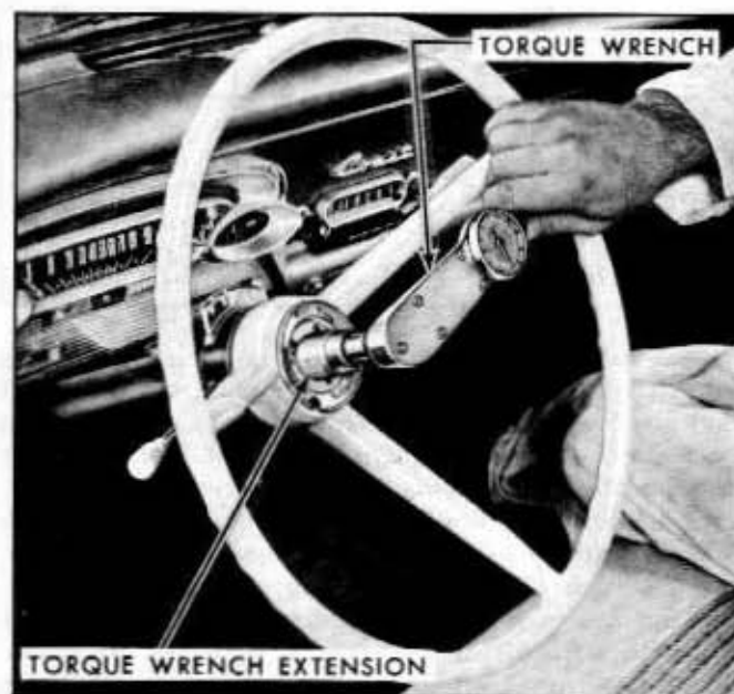
Fig. 3B-3—Steering Gear Load Check Using Torque Wrench—(60C-1203)
