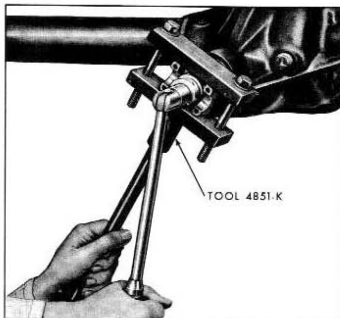
Fig. 4-8—Drive Pinion Flange Removal—(60C-5214)
