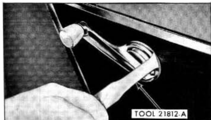
Fig. 13D-2—Handle Removal — Typical—(60C-8001)
